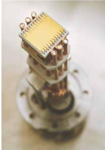
Figure 2: Atom chip for atomic micromanipulation via magnetic fields [3].
