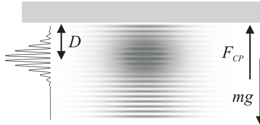
Figure 3: Sketch of the proposed experiment: an ultracold sample of atoms is trapped in a vertical optical lattice in proximity of a dielectric surface and performs Bloch oscillations under the combination of gravity and of the Casimir-Polder force.
